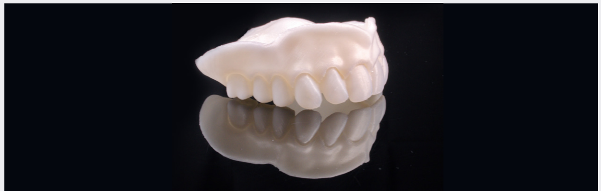
An example of trial denture 3D printed by means of fused deposition modeling technology.
