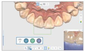
Automatically filter the color out during scanning, reducing the number of artifacts and making retraction easier.
