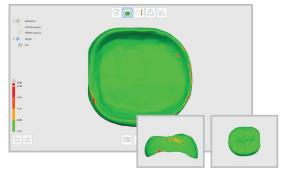
Conduct a modeless crown fitting. The software can reveal where alterations may be needed.
