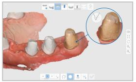
Choose between allowing the system to automatically generate the margin line for any tooth or create it manually.
